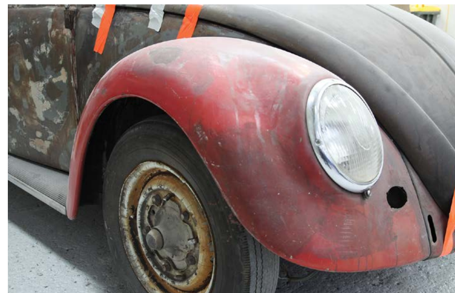
Dodgy red respray is one of a number of past "fixes" applied to this car.
